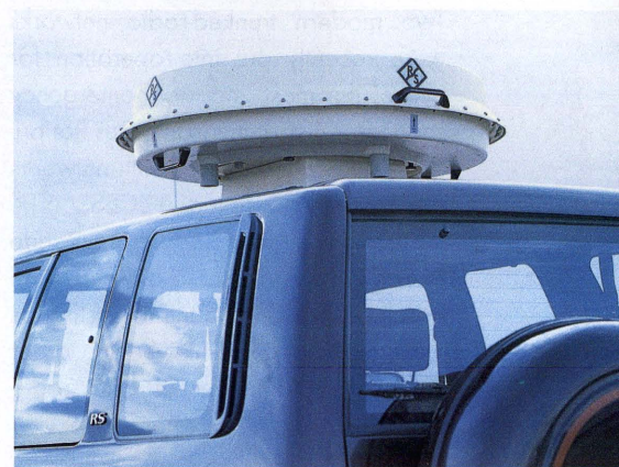
FIG 2 New antenna for mobile VHF-UHF Direction Finder PA1555 is accommodated in plastic housing with diameter of 1.1 m and height of 25 cm and covers whole frequency range from 20 to 1000 MHz. Photo 41 951/1
