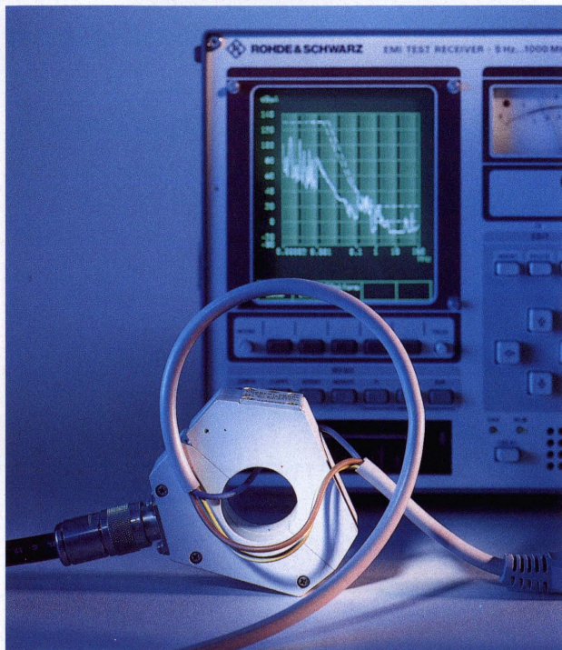
FIG 1 RF Current Probe EZ-17 for emission and bulk-current injection measurements in frequency range 5 Hz to 100 (200) MHz Photo 42 021/1
